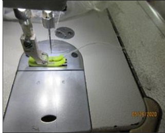
External photo(s) of the production unit(s) 7.17 No needle guard.jpg
